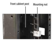
**6** Attach one mounting nut to each of the two back cabinet posts where you plan to install the server.
